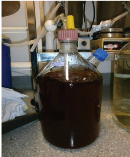
Fig. 1. Immobilization of Acidithiobacillus sp. 13 Zn and L. ferriphilum CC on zeolite (37°C, stirring through blowing)
